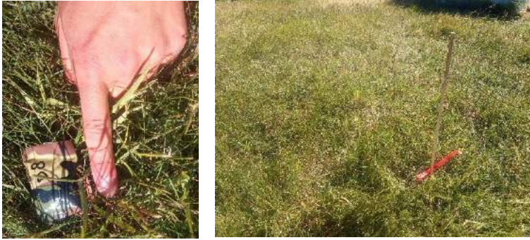
Figure 3: Size and marking of climate loggers that we will place during the experimental period. The marking sticks are ca 30 cm high.
