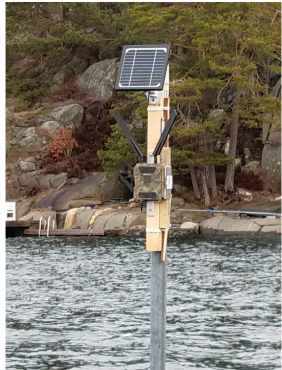
Figure 5. Time-lapse camera used in Lyngør. It consists of a solar panel placed on top and the camera with two antennas above the camera. The same setup is used at location two. Photo credit: Elsa van Meurs.
